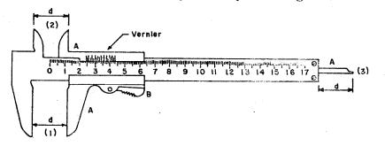
Fig. 2.2. Vernier callipers. The parts marked A form a rigid unit, which is free to move relative to the rest of the instrument when the spring-loaded button B is pressed. The three distances marked d are equal and are read off from the vernier scale. (1) gives the diameter of a rod. (2) the diameter of a hole and (3) the depth of a blind hole.
