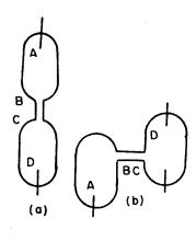
and a diameter of about one millimetre. Two aluminium or platinum electrodes are sealed into this tube at the two ends A and D (Fig. 5.45 a). The tube is filled with the gas, whose spectrum is to be studied, at a pressure of 1 or 2 mm of mercury. More than 2000 volts potential is applied between the electrodes with the help of an induction coil high tension D.C. source (power pack).
