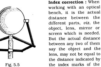
vertical stands carrying them. In order to find the actual distance, a correction known as *index correction* must be carried out in all optical experiments using an optical bench. The procedure for index correction is as follows :
