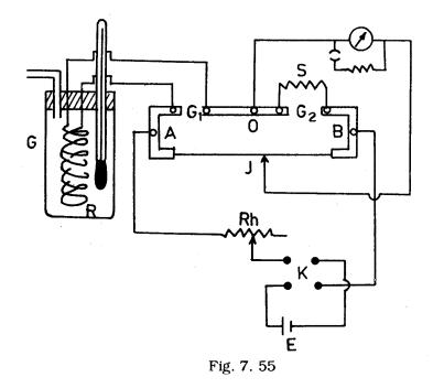
mica frame and immerse it in a glass tube G containing oil. Close the glass tube with a cork and through a hole in it, insert a thermometer. Insert the tube with its contents inside a hypsometer through an opening in the cork at its top.
