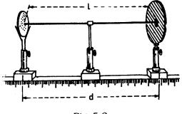
If the object or the screen or the lens is shifted to another position on the bench, the index mark moves through the same distance as the object or the screen or the lens since they are
