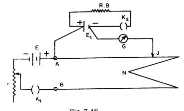
Fig. 7.48 open and closed circuits and b is the internal resistance of the cell, we have  $b = \frac{E - e}{i}$  where *i* is the current flowing through the circuit when the key K<sub>2</sub> is closed. Again  $i = \frac{e}{R}$
